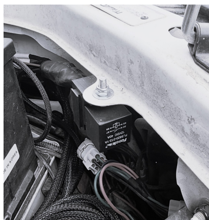
Fig. 3 Relay mounting location
